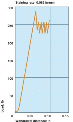
Figure 15: Pull out characteristic for single wire embedded in polyester resin/ silica.
