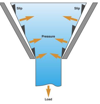
Figure IV: Load causes the cone to slip at the socket interface and the pressure generated locks the cone within the socket.
