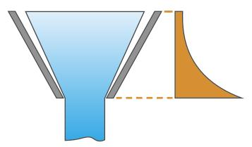
Figure V: Distribution of pressure on the cone within the socket.
