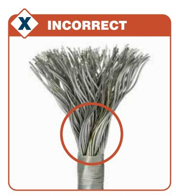
Figure 4: Incorrectly broomed wire rope.
