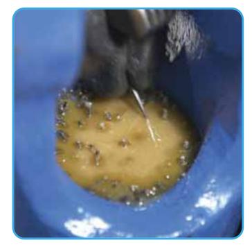
Figure 11: Scratch testing the material in the socket one hour after it has gelled.
