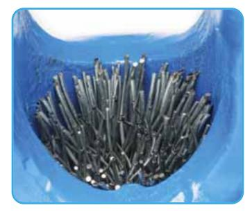
Figure 5: Properly positioned broom with the wire ends protruding slightly.
