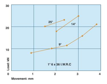
Figure II: Movement within the socket under load for the two extreme angles & the standard 14° taper.
