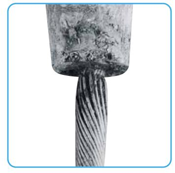
Figure 13: Typical example of the swelling of stainless steel rope due to Crevice Corrosion.
