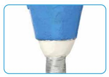
Figure 7: Axes of socket and rope properly aligned and sealed with WIRELOCK putty/ clay.
