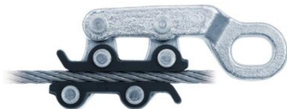
These wire grips are the ideal tool to safely tensioning of copper and steel cables. They have a wide range of applications in manufacturing, agriculture and bridge construction. The profile of the clamping jaws is specifically designed for copper and steel cables so that the stretched material does not become damaged.
