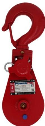
The POWERTEX PSBH-S2 snatch block with hook is a heavy-duty snatch block that can be used for temporary or permanent lifting and pulling installations. The block can be used to redirect a wire rope or increase the load that a wire rope winch arrangement could handle in a straight loading without a block.
