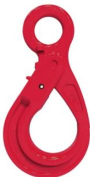
The POWERTEX Self-Locking Hook with eye is part of the Powertex G10 Lifting Sling Chain Components range. The self-locking hook closes and locks itself when lifted, making it a safe lifting hook. The hook can be opened by pressing the pawl on the back of the hook. The latch can not be removed.
