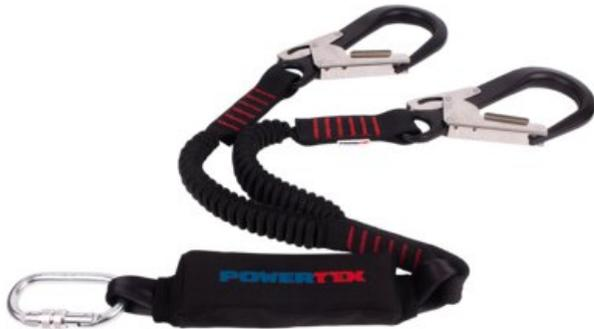
The Powertex FL-2 double-leg flexible lanyards are equipped with a shock absorber and approved for 140 kg use. These lanyards have an elastic quality that allows them to stretch in accordance with the user's movements. Both lanyards are securely sewn to a shock absorber pack, which includes a screw gate steel carabiner for attachment to a harness. On the other end of the lanyards, sewn-in double-action aluminum scaffold hooks provide reliable anchorage.
