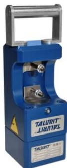
The Talurit® 22T 1P swager has a single pillar open throat design and is coupled with an efficient hand pump for high mobility. Thanks to its low weight and easy operation, it is just as convenient to use in the field as in the workshop. The reliable hydraulic hand
